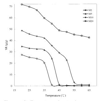
**Figure 5** Swelling ratios as a function of temperature for various NIPAAm-co-SA50 gels in deionized water.
