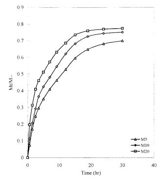
**Figure 10** Phenolphthalein release profile for NIPAAm-*co*-SA50 gels during swelling at 25°C and deswelling at 50°C under pH 11 buffer solution.
