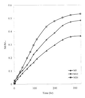
**Figure 8** CV release profile for NIPAAm-*co*-SA50 gels during deswelling at 50°C.
