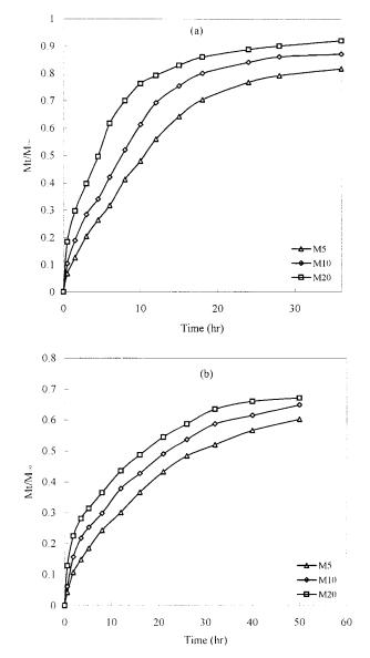
**Figure 9** Phenolphthalein release profile for NIPAAm-*co*-SA50 gels (a) during swelling at pH 5 and deswelling at pH 11 (37°C) and (b) during swelling at pH 9.02 and deswelling at pH 2.24 (37°C).
