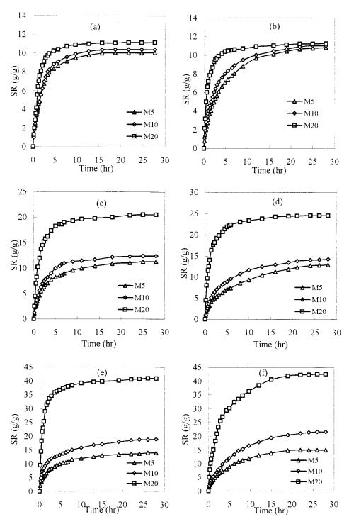
**Figure 1** Swelling ratios as a function of time for the series of NIPAAm-*co*-SA50 gels at 25°C under pH (a) 2.244, (b) 4.13, (c) 6.05, (d) 7.96, (e) 9.02, and (f) 10.64.
