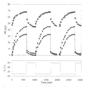
**Figure 6** Swelling ratios of NIPAAm-*co*-SA50 gels as a function of time repeated abrupt change of temperature between 25 and 55°C in deionized water: ( $\triangle$ ) M5; ( $\Diamond$ ) M10; ( $\Box$ ) M20.
