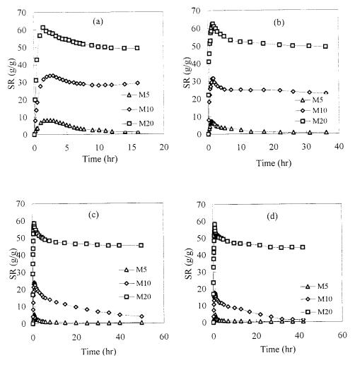
**Figure 4** Swelling ratios as a function of time for the series of NIPAAm-*co*-SA50 gels in deionized water under (a) 45, (b) 50, (c) 55, and (d) 60°C.
