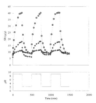
**Figure 7** Swellings ratios of NIPAAm-*co*-SA50 gels as a function of time repeated abrupt change of pH between pH 2.24 and 9.02 in buffer solution at 25°C: ( $\triangle$ ) M5; ( $\bigcirc$ ) M10; ( $\square$ ) M20.
