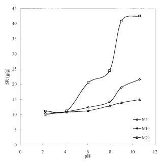
**Figure 2** Swelling ratio as a function of pH value for the series of NIPAAm-*co*-SA50 gels at 25°C.
