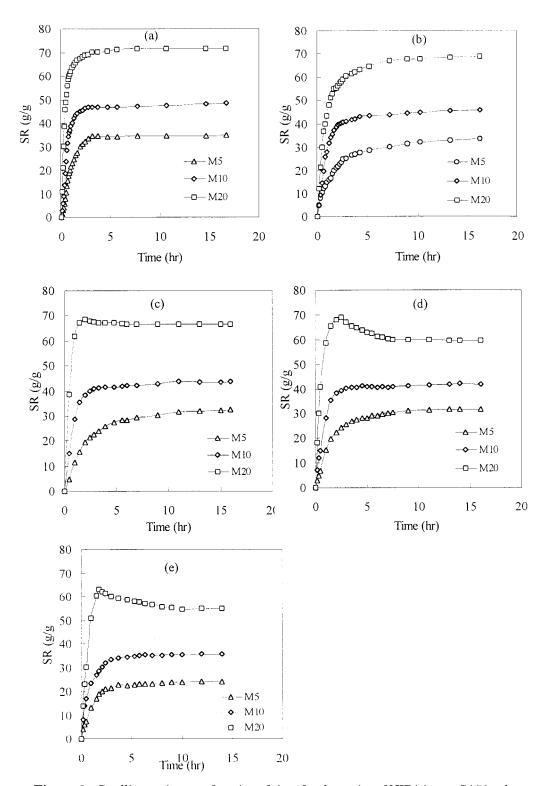
**Figure 3** Swelling ratios as a function of time for the series of NIPAAm-*co*-SA50 gels in deionized water under (a) 20, (b) 25, (c) 30, (d) 35, and (e) 40°C.
